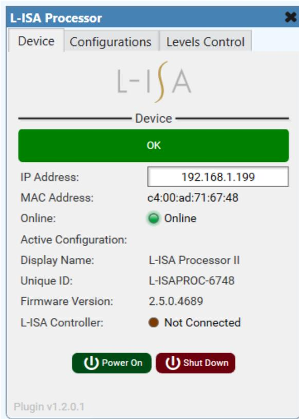
The Device tab displays general information about the connected L-ISA Processor and its current status.
